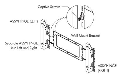
2 After installing the Wall Mount Bracket, assemble the support bars and hinges (as illustrated) using screws provided. (12 screws(2) are provided. For safety reasons, make sure all 12 screws are firmly attached.)
